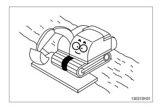
wood boards on the ground to prevent the machine sinking.
